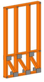
PSP™ Parapet Shear Panel
